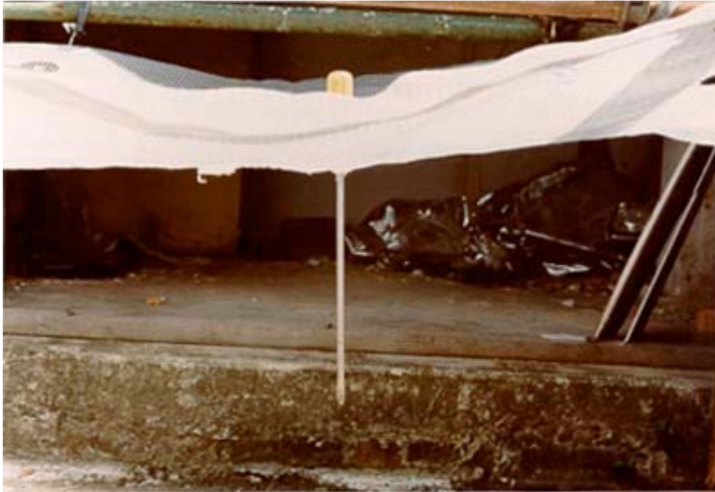
Photograph 2. Sheeting pierced but not penetrated by a 300mm screwdriver of 280gm weight.
